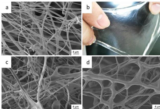
*Figure 4 SEM micrograph of PASP-DAB fibers (a), picture taken of a PASP-CYS membrane (b), SEM micrographs of PASP-CYS (c) and PASP-THD-PEO fibers (d)*
