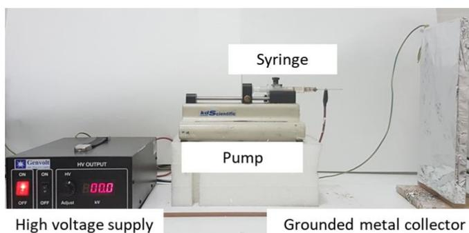
*Figure 2 Setup of electrospinning machine*
