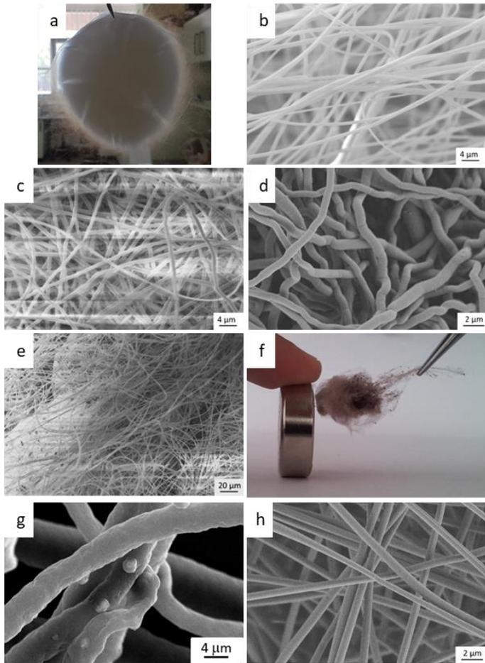
*Figure 3 Electrospun PSI fiber membrane (a) fibers (b); PSI-DAB fibers (c), PSI-THD fibers (d), PSI-CYS fibers (e), magnetic particle loaded PSI-CYS fiber membrane attracted by magnet (f) and a SEM micrograph of the same sample (g) PSI-THD-PEO fibers (h)*
