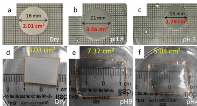
*Figure 5 Dry PSI fibrous membrane (a), PSI-DAB in pH 8 buffer solution (b) and in pH 3 (c), PSI-THD-PEO membrane (d), PASP-THD-PEO membrane in pH 9 (e) and in pH 4 buffer solutions (f)*
