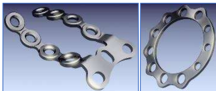
Figure 31. - Planned modifications - bending and beveling of the plate, increasing the ring hole - FCA
